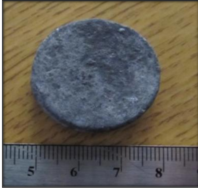
Figure 24: The \text{SiO}_2 coated over \text{NaNO}_3 pellet
