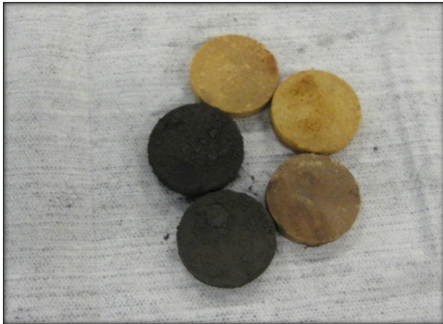
Figure 23: Polymer and Ni-polymer coated and cured pellets
